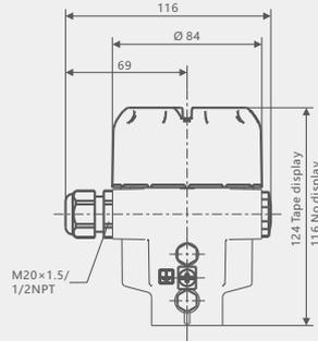
Single chamber housing, forged stainless steel
