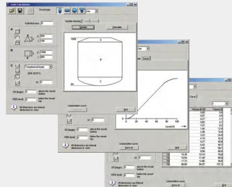
For HART output signals, Profibus-PA and FF, DTM can be used according to the FDT standard. For all transmitter setup and control procedures, DTM provides a self-parsing, clear user interface. When testing, DTM also simulates all process values and archives parameter data. Measurements can be recorded for diagnostic purposes.
