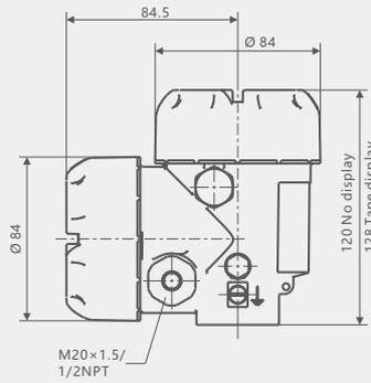
Double chamber housing, forged stainless steel
