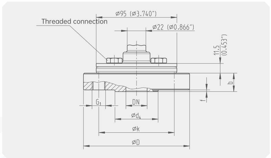
**Flange connection, according to ASME B16.5 standard (sealing surface: RF 125... 250 AA)**
